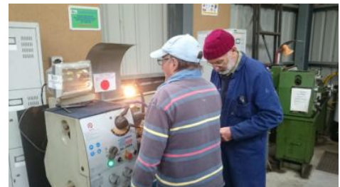
Derrick Conry showing a member how to use the metal lathe with the digital read-out [the latter purchased through a grant from the Department of Premier and Cabinet (DPAC) in conjunction with the Tasmanian Men's Sheds Association (TMSA)]
